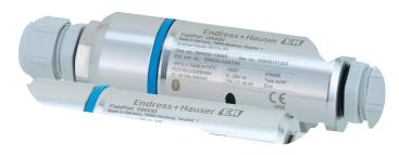
The FieldPort SWA50 converts the HART signal of the connected HART field device to a reliable and encrypted Bluetooth® or WirelessHART signal. The Endress+Hauser SmartBlue app or the Endress+Hauser Field Xpert can be used to configure the FieldPort SWA50. Remote configuration via the DTM using WirelessHART network is also possible.
