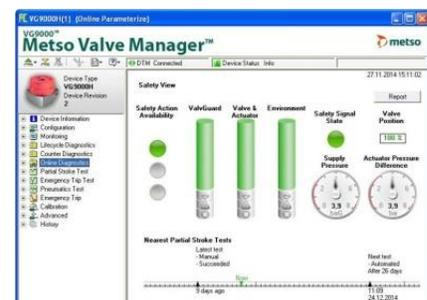
This DTM by Metso provides an easy to read graphical interface to help you migrate to a predictive maintenance
