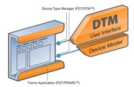
Figure 4: Within the FDT ecosystem, the FDT/FRAME can be embedded in standalone device management tools.
