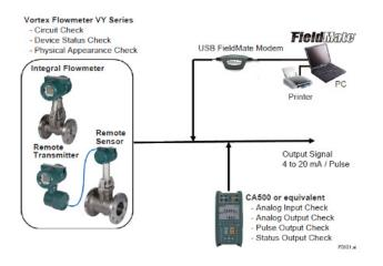
Fig. 6 System configuration
