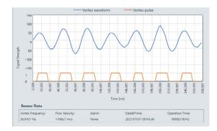
Fig.4 Screen of waveform monitoring for FSA130
