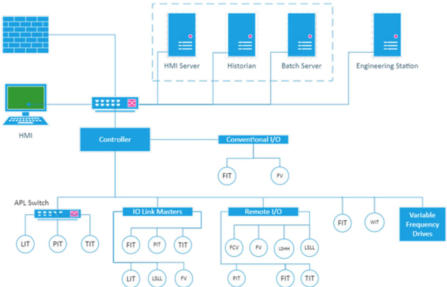
Figure 2: The SPC Today migrated to include APL and added IO-Link to its EtherNet/IP architecture.
