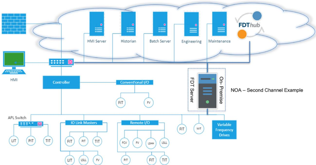
Figure 5: SPC Future Networks and Architectures with NOA second channel FDT Server on-premise with online cloud access to the FDT hub. The solution allows monitoring and optimization of all field devices via OT and IT clients with all services hosted in the cloud.
