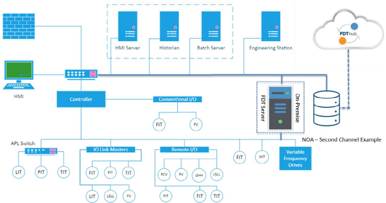
Figure 4: SPC Today with NOA second channel FDT Server on-premise with a local copy of the FDT hub. The solution allows monitoring and optimization of all field devices via OT and IT clients with all services hosted on-premise.
