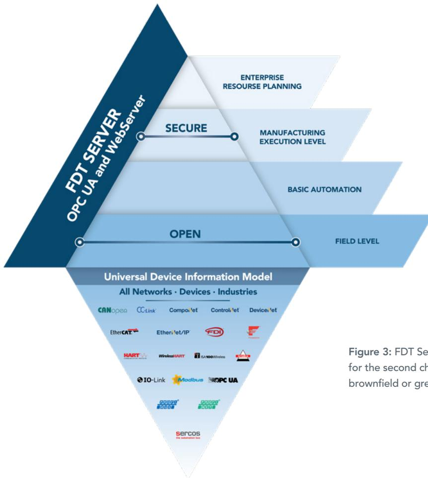
Figure 3: FDT Server architecture based on NOA-175 recommendation for the second channel provides an open and secure connection to brownfield or greenfield architectures.
