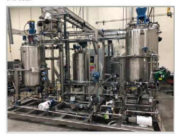
Figure 1: P&G's Ethernet-APL demonstration project at the company's Corporate Engineering Technology Lab (CETL) in West Chester, Ohio. This includes four tanks from 375 to 500 kg, six pumps with flowmeters, and three units performing continuous and batch operations. It runs water as its process fluid and is completely self-contained and remotely operated.
