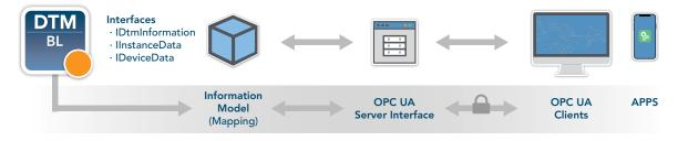
Figure: FDT DTMs expose device-specific data via information mapping to authenticated OPC UA Clients and customized apps.
