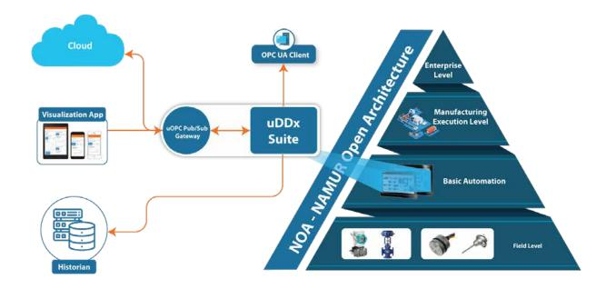
uDDx Suite polls the network topology of automation systems and reads the Device Identification, Device Diagnostics, Process Values, and Device Core Parameters using uDDx Suite's interpreter DTM component. The OPC UA component of uDDx Suite uses this data to construct OPC UA information model according to the PA-DIM standard.
