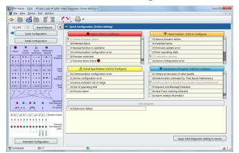
Configuration and confirmation of device alarms conforming to NE107 Field Diagnostics can be implemented intuitively on the graphical display.
