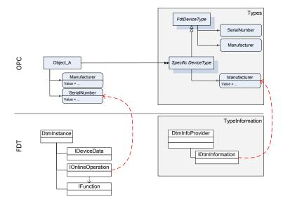
Fig.4 Mapping of device type information [5]
