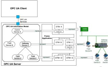
Fig.2 OPC UA architecture according FDT2.0 [3]
