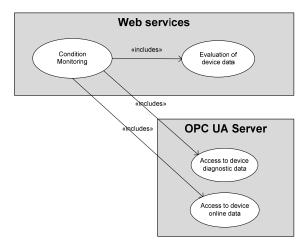
Fig.3 Use case "Condition monitoring"
